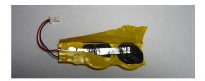
3. Then enclose the entire yellow cover tightly, firmly with adhesive tape, you can also verify whether they are at right position because the yellow cover is semi transparent.
